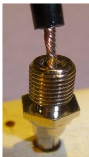
Fig. 6 - 18 Ga. Fig. 7 – Alligator crimped on the wire not the insulation.
