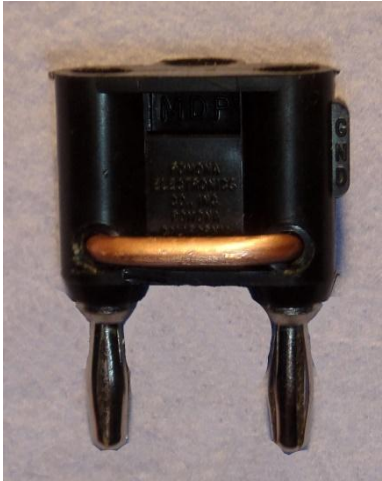
Fig. 14 – 3/4” Adapter made into a low resistance “short.”
