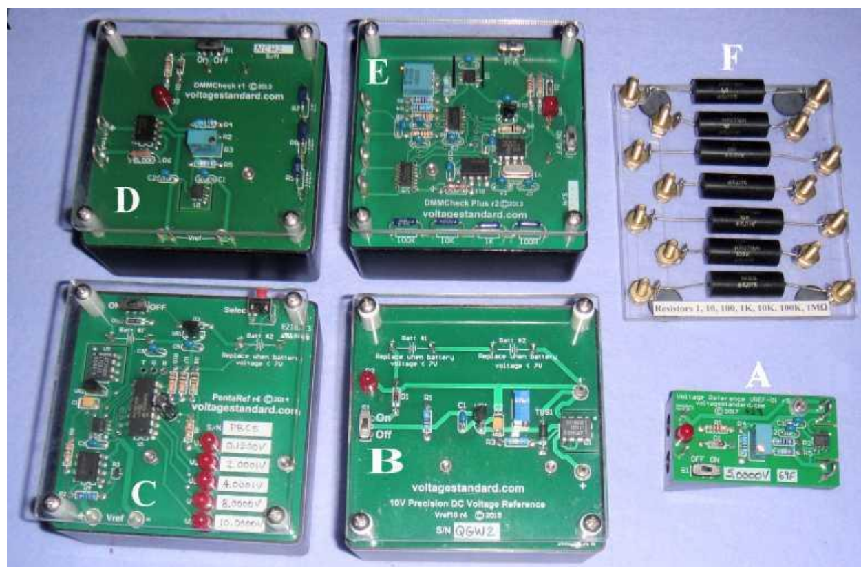
Fig. B1 - AC & DC voltage, current & resistor standards (A – E) and DMM 1W standard resistors (F). See text.
