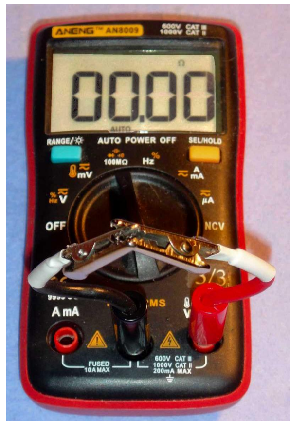
Fig. 10 – AN8009 DMM does not show the lead resistance with 0.01 ohm resolution, lead set #4.
