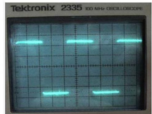
Fig. 3 –DMMCheck Plus AC voltage wave form.
