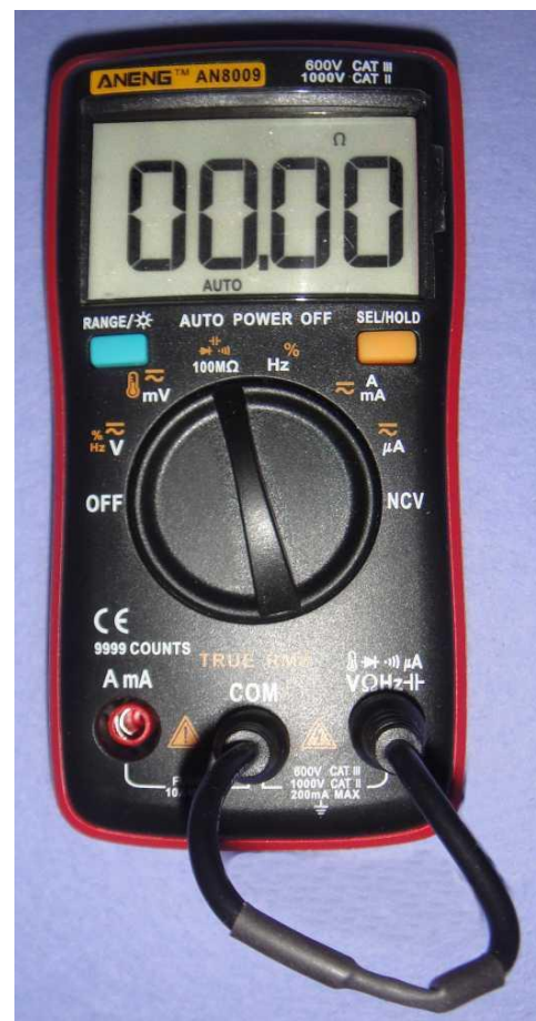
Fig. C3 - Testing 6" universal test leads.
