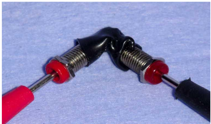
Fig. 5 – Proper test lead connection for “shorting”
