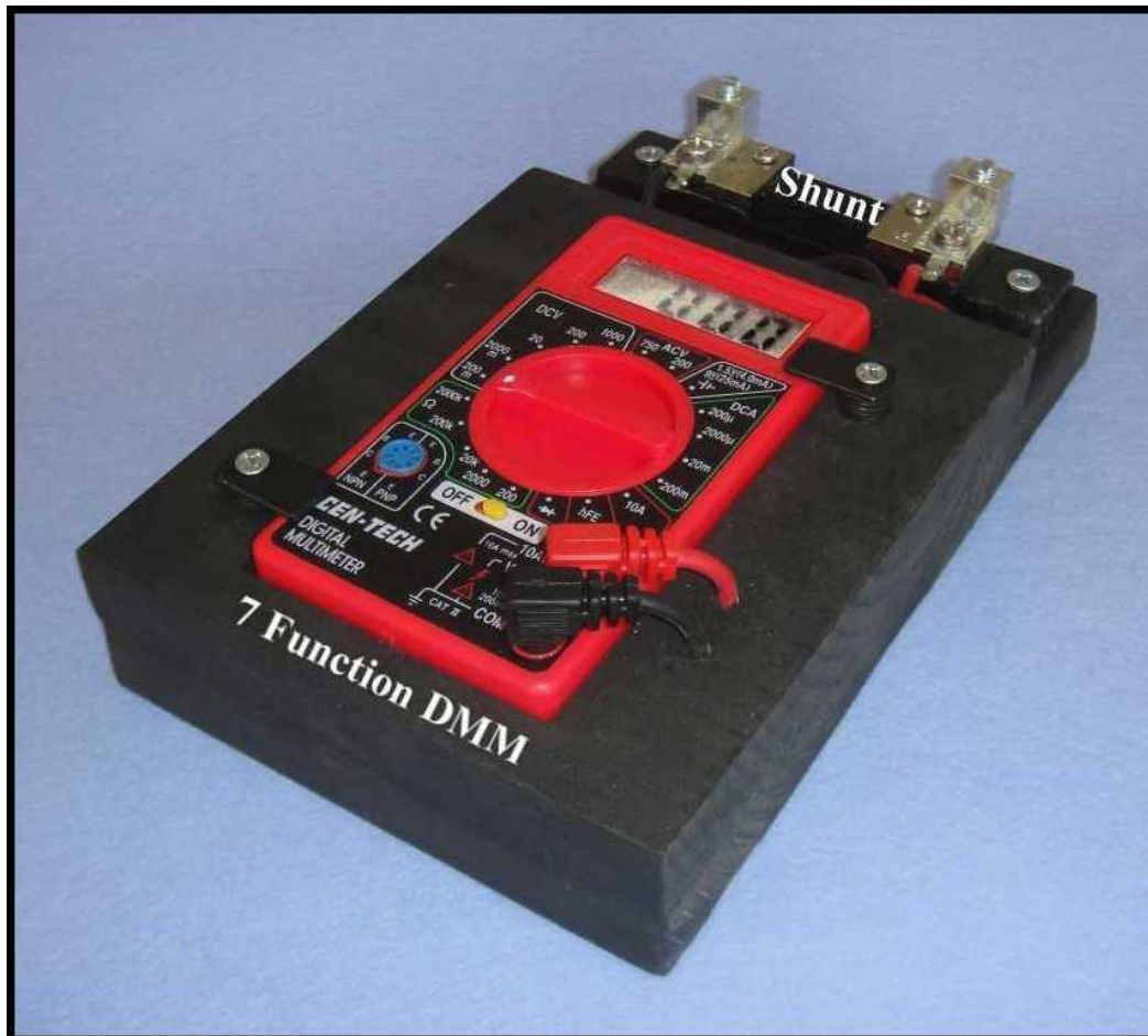
Fig. N2 – A 7 Function DMM is used to display the millivolts from a 50-ampere shunt in this DIY writing project.
