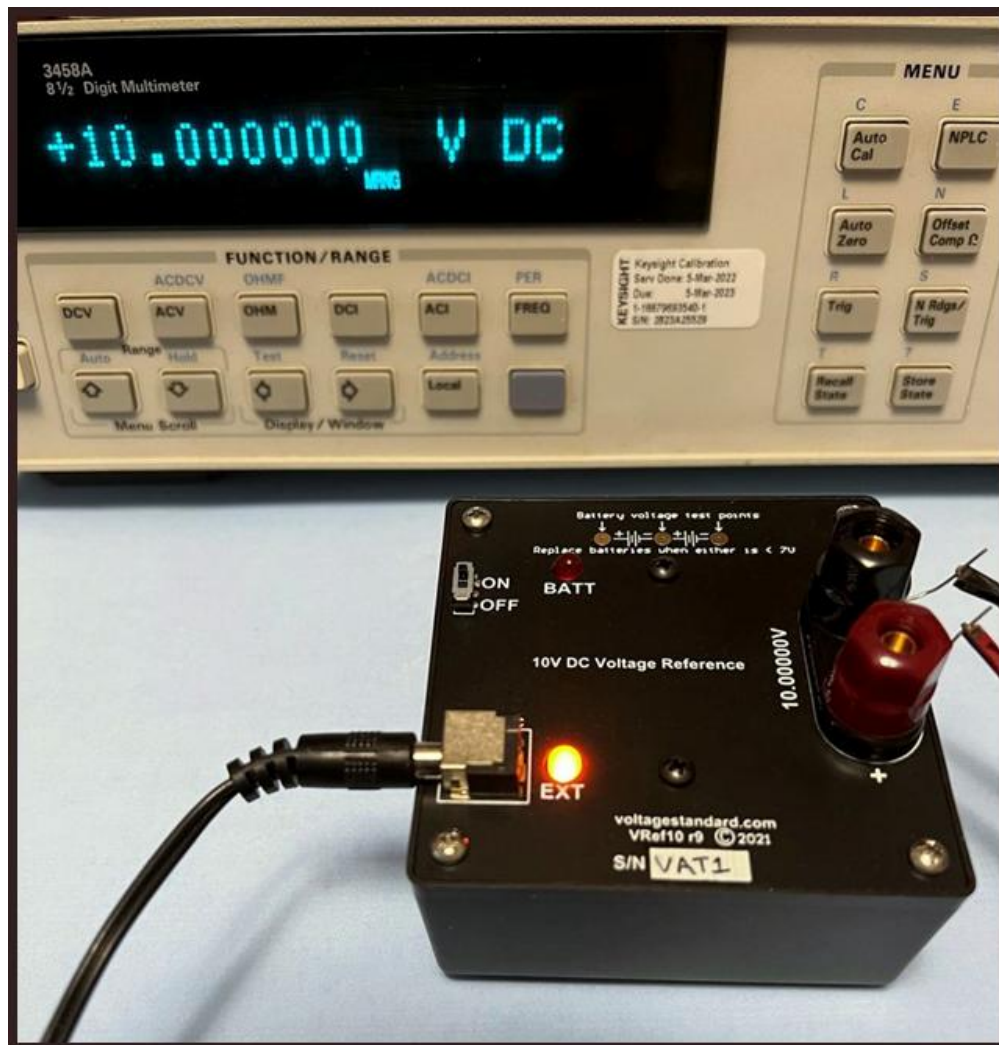
Fig. II – NIST 8-1/2 digit meter used to set the VREF10-001 r9.
