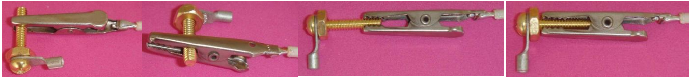
Fig. 8a - Side normal. Resistance = 4.7 mΩ. Fig. 8b - side normal deep. Resistance = 2.5 mΩ. Fig. 8c – End normal. Resistance = 3.0 mΩ. Fig. 8c – End deep. Resistance = 2.7 mΩ.
