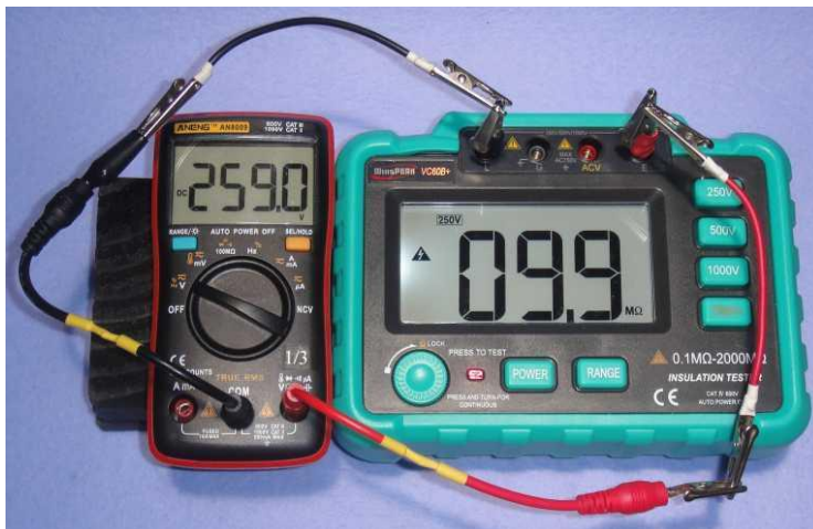
Fig. F3—This meter measures a correct ( \approx low) 10 M \Omega R_M .
