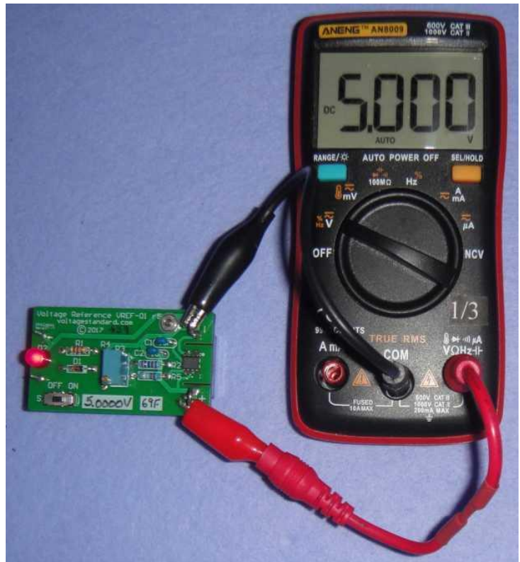
Fig. 1 - ENEG AN8009 DMM measuring a 5-volt standard.
