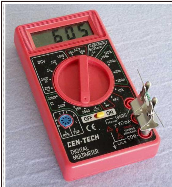
Fig. 10 – Low cost DMM with close test jacks.
