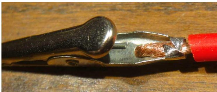
Fig. 6 - 18 Ga. Fig. 7 – Alligator crimped on the wire not the insulation.
