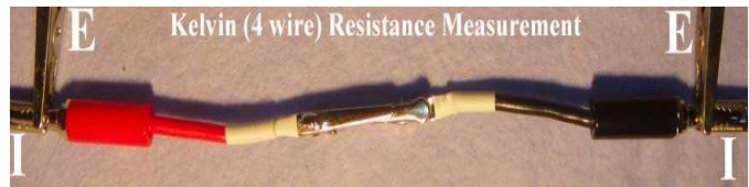
Fig. 11 – Kelvin 1A connection to measure test leads.
