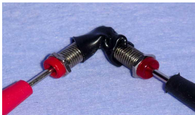
Fig. C5 – Back-to-back pin jacks are the best for shorted test lead resistance measurement.
